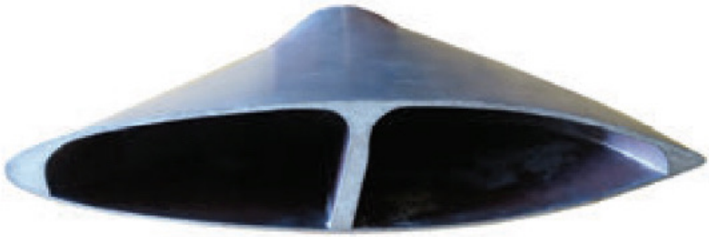
Figure 2-8. Cross section of steel propeller blade.
