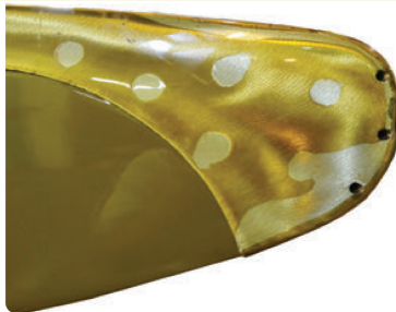
Figure 2-5. Tip on wooden propeller revealing soldered attachment hardware and drain holes.
