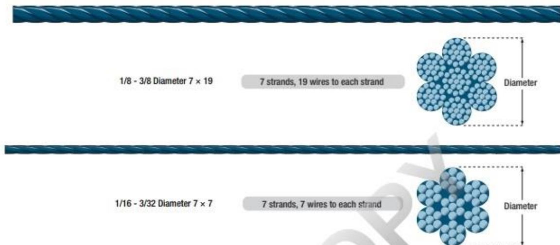
Figure 10-1. Cable cross sections.
