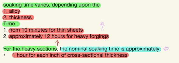
Choose the minimum soaking time necessary to develop : the required physical properties
