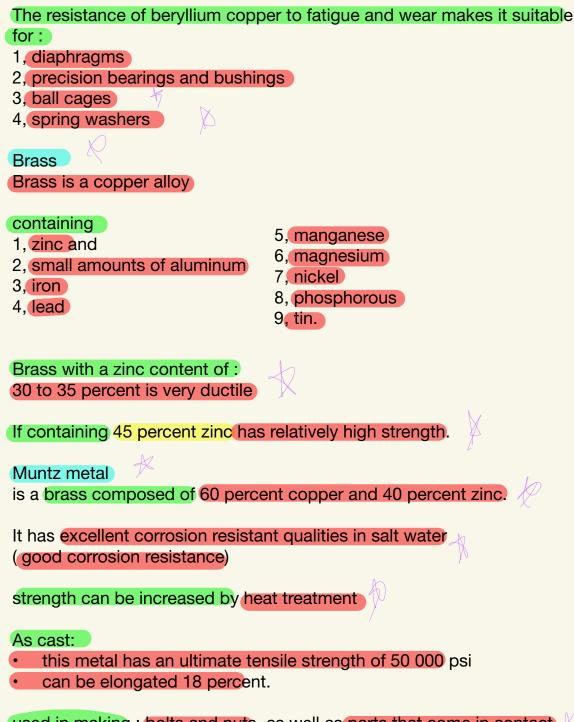
used in making : bolts and nuts, as well as parts that come in contact with salt water
