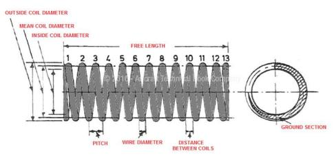
spring includes a number of coil turns but does not include any end treatment such as an eye or hook used as an attach point.
