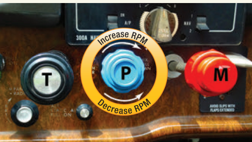
Figure 3-2. Push-pull type controls for throttle (T), propeller (P),
