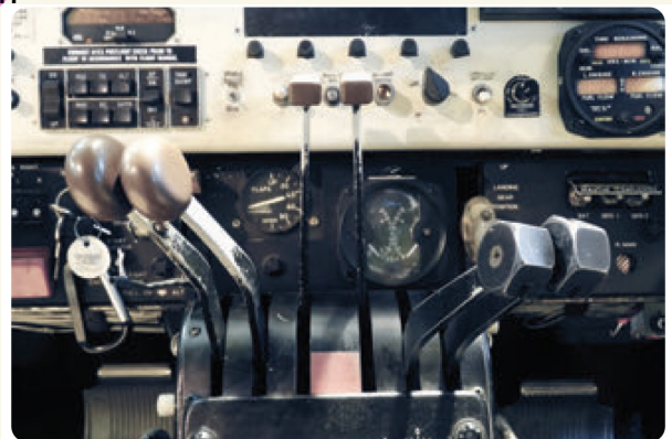
Figure 3-1. Throttle; propeller; and mixture controls of twin engine aircraft.
