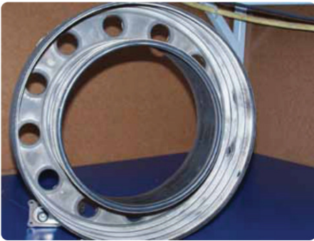
Figure 5-6. Annular combustion with chamber ceramic coating.
