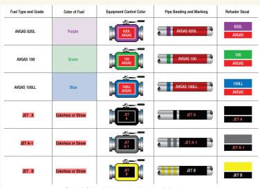
Figure 9-2. Color coded labeling and markings used on fueling equipment.
