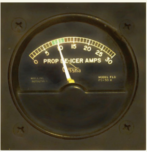
Figure 5-9. Propeller de-icer ammeter. Heating elements should draw green arc current.
