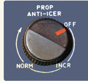
Figure 5-11. Rheostat control on anti-ice with variable flow.
